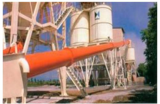
Magnetite Iron Sand processed from siphon vessel to export cargo vessel is by pipe conveyor (as shown in photo), the magnetically separated sand is still with high moisture content. Hence, no dust can be produced during the transfer operation.
